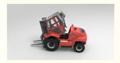
GOODSENSE 3.5 TON 4 WHEEL DRIVE ROUGH TERRAIN FORKLIFT IS A VERY STRONG FORKLIFT DESIGNED FOR MAXIMUM PERFORMANCE UNDER THE MOST DEMANDING CONDITIONS. THANKS TO ITS GROUND CLEARANCE, ITS FOUR LARGE WHEELS AND 4×4 DRIVE, IT MOVES SWIFTLY ACROSS MUDDY OR ROCKY TERRAIN AND OVERCOMES OBSTACLES SUCH AS ROCKS, KERBS AND POTHOLES WITH EASE. TRACTION CAN BE CHANGED FROM 4×4 TO 4×2 BY A SWITCH WITHOUT STOPPING THE VEHICLE WHEN MOVING ONTO BETTER TERRAIN, THEREBY SAVING FUEL.
